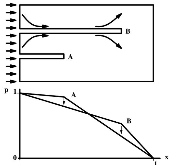
**Figure 3.** Two dissolution channels in the fracture (top) and the corresponding pressure drops (bottom). The flow lines are converging toward a larger channel at the inlet and diverging near the tip of the conduit.
