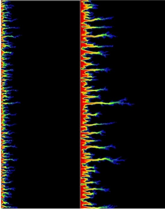
**Figure 1.** Aperture growth due to dissolution in an artificial fracture at  $Pe = 8$ . The figure shows dissolution patterns at (left)  $\Delta h = 0.15h_0$  and (right)  $\Delta h = 0.5h_0$ . The colors indicate regions of low (blue), medium (green), and high (red) aperture growth. The flow direction is from left to right. Only 1/3 of the fracture (the leftmost part) is shown.
