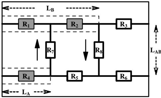
**Figure 4.** A resistor network corresponding to the configuration of Figure 3. The arrows denote the directions of the currents between the channels.
