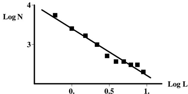
**Figure 2.** The cumulative distribution  $N(L)$  of channel lengths in the fracture simulated with the pore scale model ( $Pe = 8$ ). The solid line has a slope of  $-1.2$  and all logarithms are natural.
