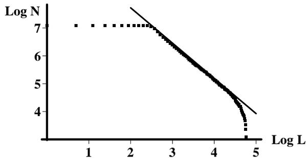
**Figure 6.** The cumulative distribution  $N(L)$  of channel lengths from in the fracture simulated with the resistor network model. The solid line has a slope of  $-1.25$ .
