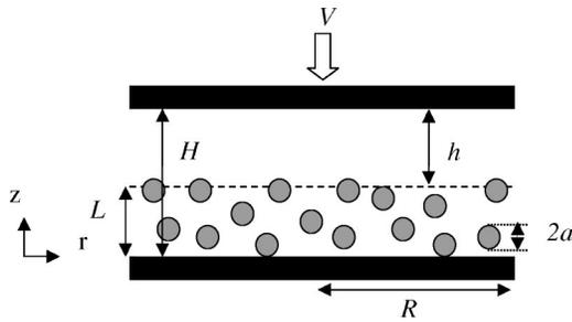
FIG. 1. Sketch of the geometry used in the simulation. The figure is a side view of a squeezing flow geometry using two flat disks of radius  $R$ , separated by a distance,  $H$ . The upper surface is moving downwards with a velocity  $V$ . The lower surface is stationary and coated with a suspension of either fixed or mobile beads of radius  $a$ . The thickness of the coat is  $L$ .
