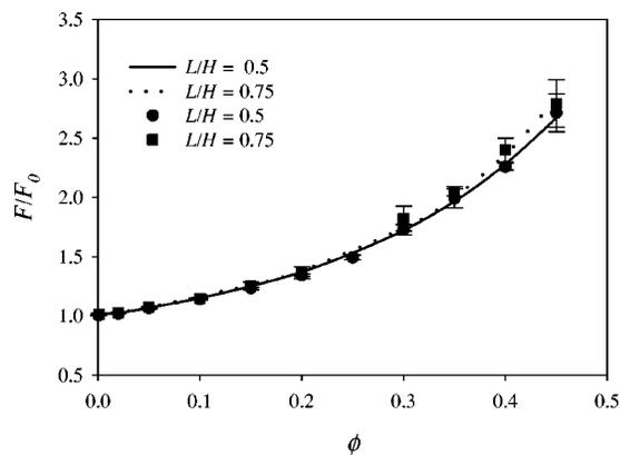
FIG. 6. Lubrication force for immiscible viscous fluids in a system of height  $H=50\Delta$  and  $R=75\Delta$ . Lattice-Boltzmann simulations of the lubrication force (symbols) are compared with theoretical calculations based on the Stokes equations using the high-frequency viscosity,  $\eta_\infty(\phi)$  for each region (see text).
