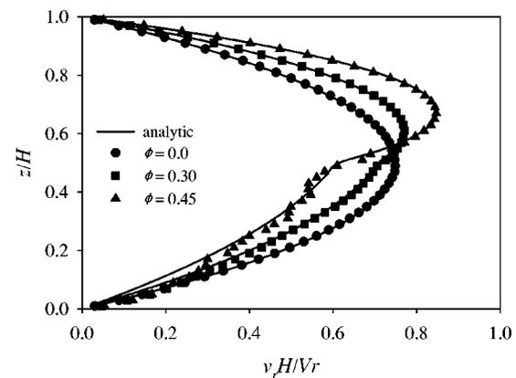
FIG. 7. Radial flow field for a two-phase viscous flow ( $L/H=0.5$ ). The dimensionless radial velocity  $v_r(r,z)H/Vr$  was averaged over radial direction and plotted as a function of  $z$ . For a radially homogeneous incompressible flow  $v_r \propto r$ . Lattice-Boltzmann results at different volume fractions (solid symbols) are compared with analytic solutions (solid lines) using the effective viscosity of the medium (Ref. 21).
