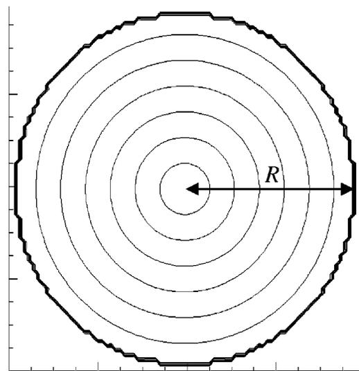
FIG. 2. Contour plot of the radial velocity field in the horizontal plane at  $z=H/2$  for a single phase flow. The equally spaced contours show that the radial velocity increases linearly with the radial distance, which follows from the incompressibility of the flow. The smooth circles show that the effect of the pixelated outer surface do not penetrate into the flow.
