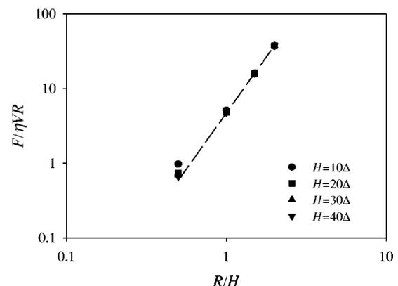
FIG. 3. Dimensionless lubrication force ( $F/\eta VR$ ) as a function of the aspect ratio  $R/H$  for different heights. Analytic calculations indicates a power law dependence proportional to  $(R/H)^3$  as indicated by the dotted line. The simulation results are within 1% of the analytic prediction when  $R > 1.5H$ .
