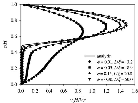
FIG. 9. Radial flow field for a squeezing flow including a porous matrix ( $L/H = 0.5$ ). The dimensionless radial velocity  $v_r(r, z)H/Vr$  was averaged over radial direction and plotted as a function of  $z$ . Lattice-Boltzmann results for different screening lengths (solid symbols) are compared with analytic solutions (solid lines) using the effective permeability of the medium  $K = \xi^2$  (see Appendix C).
