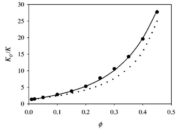
FIG. 5. Inverse permeability of a random array of solid spheres. Lattice–Boltzmann simulations (circles) are in good agreement with a precise multipole solution of the Stokes equations (solid line) (Ref. 21). The self-consistent solution of the Brinkman equation for the permeability is also shown (dotted line) (Ref. 16). The lattice–Boltzmann results are the average of ten independent configurations, and the resulting statistical errors are smaller than the size of the plotting symbols.
