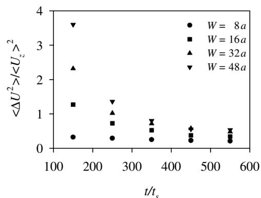
FIG. 2. Time dependence of the relative velocity fluctuations,  $\langle \Delta U^2 \rangle / \langle U_z \rangle^2$ , for four different container widths.
