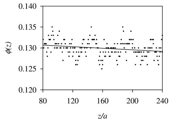
FIG. 3. Particle volume fraction as a function of height. The particle density in the viewing window ( $80a < z < 240a$ ) was averaged over the last 200 Stokes times of the simulation ( $400t_s < t < 600t_s$ ). A least-squares fit (solid line) gives a slope of about  $10^{-5}$ , corresponding to  $l \approx 13000a$ .
