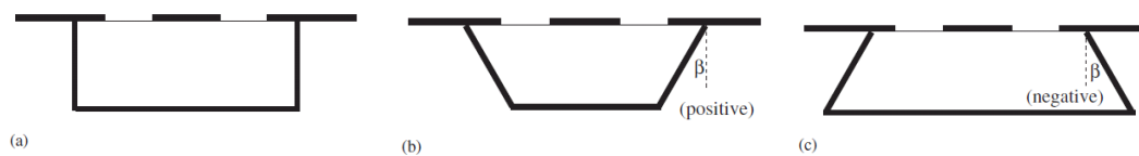
Figure 5. Etching sidewall shapes: (a) rectangular-shaped, (b) positive sloping, and (c) negative sloping [4].
