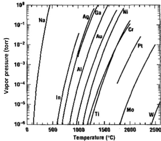
Figure 2: Vapor pressure curves for commonly evaporated materials [2].
