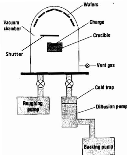
Figure 1. Schematic of an evaporator equipped with a diffusion pump [2].
