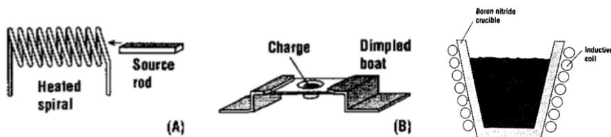
*Figure 3: Examples of evaporator systems: (A) Resistive - Simple sources include heating the charge itself and using a coil of refractory metal heater and a charge (source) rod. (B)*
