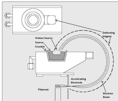
*Figure 4: Electron beam evaporation source with a 270° arc in which the beam can be led across the surface of the charge. The magnet must be much larger than shown to achieve the full 270° of arc [3].*
