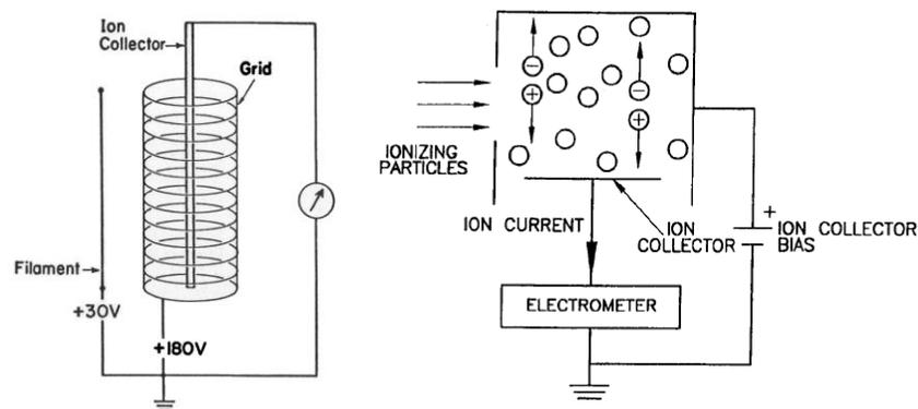
Figure 5. Schematics of an ion gauge (left). The gas molecules are partially ionized and the ions are collected by the collector (right) [6].
