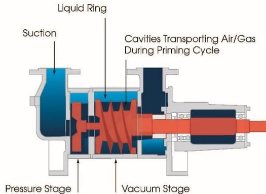
Figure 1. Schematic of a Mechanical Pump [1].
