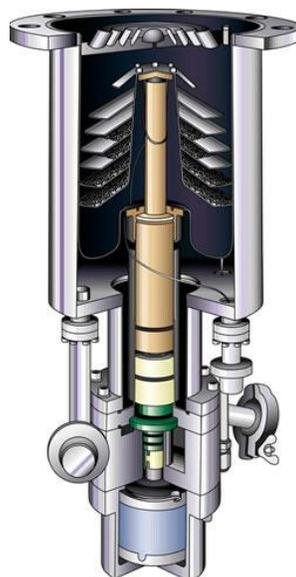
Figure 4. Cryopump [4]
