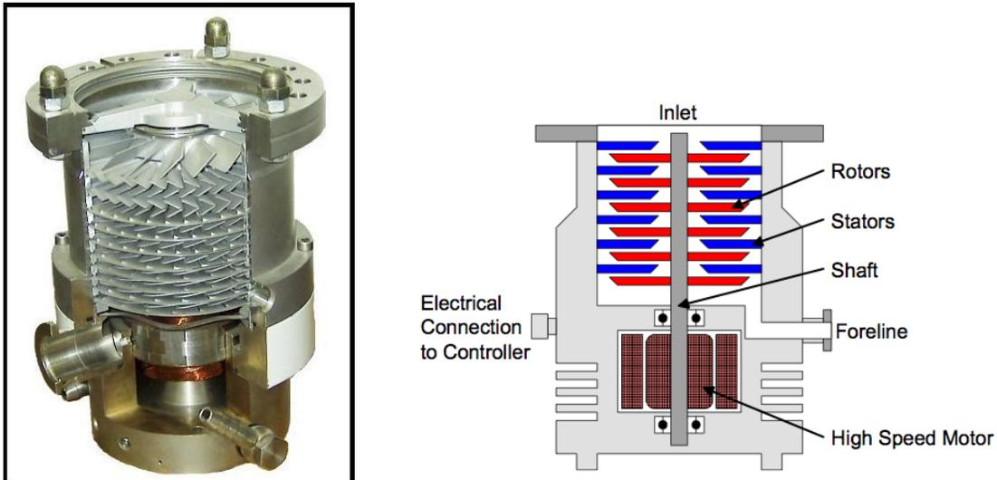
Figure 2. Turbo-molecular pump [2]
