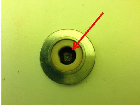
Figure 5. Spinner chuck with O-ring
