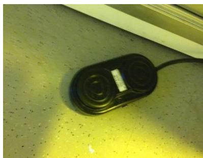
Figure 7 Foot switch for turning spinner ON/OFF
