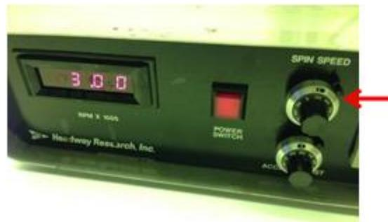
Figure 6 Spinner display indicating spin speed dial
