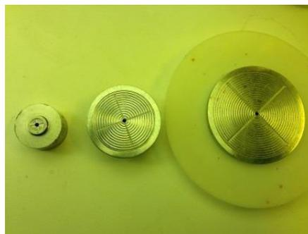
Figure 4 Different spinner vacuum chucks
