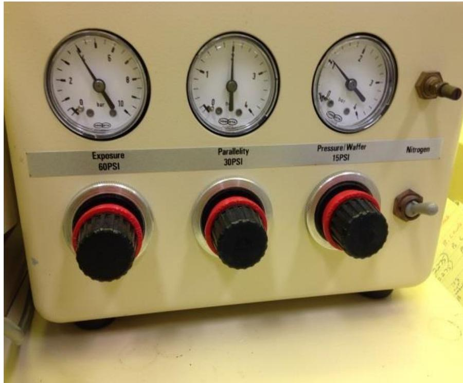
Figure 1. Pneumatics control box Pressure readings are (from left to right): 4 bar, 2 bar, and 1 bar.
