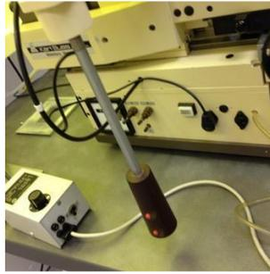
Figure 5. Microscope Joystick handle
