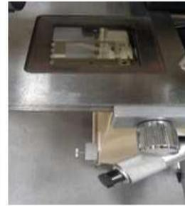
*Figure 10. Place the mask holder to the aligner*
