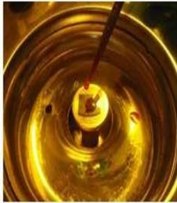
*Figure 6. Dispense the photoresist at the center of the wafer*
