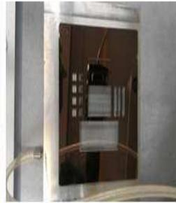
*Figure 9. Place the mask onto the mask holder*
